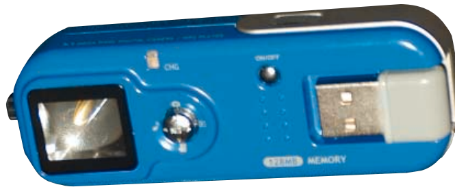
PCW featured a QVGA (320 x 240) organic microscreen from Edinburgh-based Microemissive Displays in January 2005 (page 33). It measures just 5.76 x 4.32mm and uses polymer light-emitting diodes that provide a bright, sharp image. The company displayed this prototype media player, which allows you to watch movies through a magnifying eyepiece, at the Innovations show
